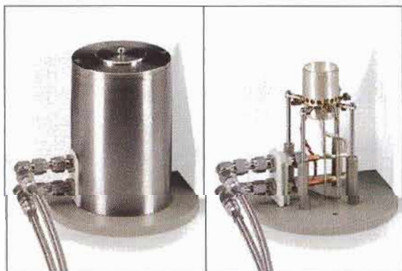
DSC 302 (-90°C – 400°C) measuring cell
