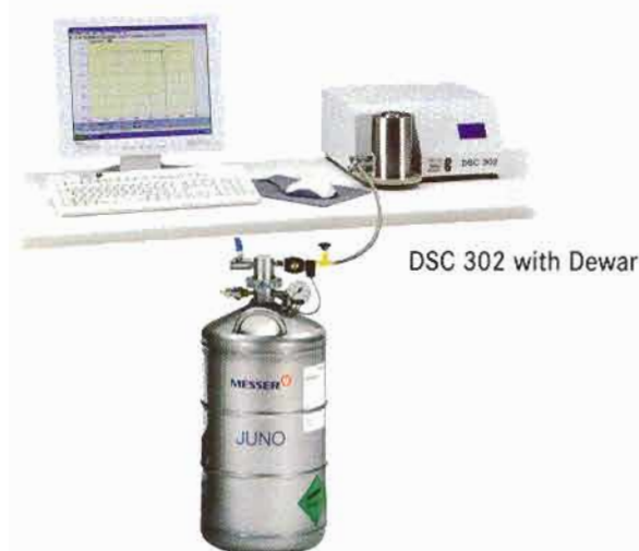
DSC 302 (-90°C – 400°C) measuring cell
